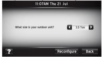
This is <u>VERY IMPORTANT</u>, you must tell the communicating control what the actual tonnage is of the equipment, failure to do so <u>WILL LOCK</u> the wrong airflow data into the system, and you WILL NOT be able to change it without replacing the outdoor control board.
